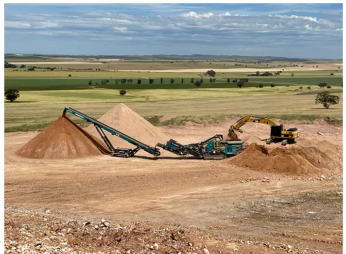
Above: crushing in Woolfords Pit for the Laura-Beetaloo Road; Below: before and after shots of Georgetown-Narridy Rd
